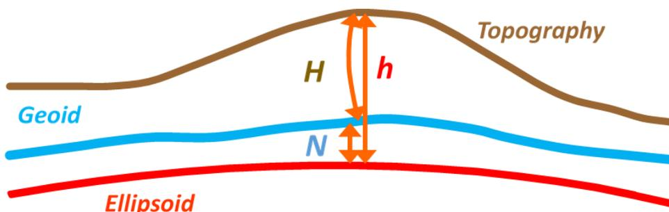
*Figure 1: Ellipsoid vs AHD Heights ( $H$  = AHD,  $h$  = ellipsoidal height and  $N$  = geoid ellipsoid separation)*
