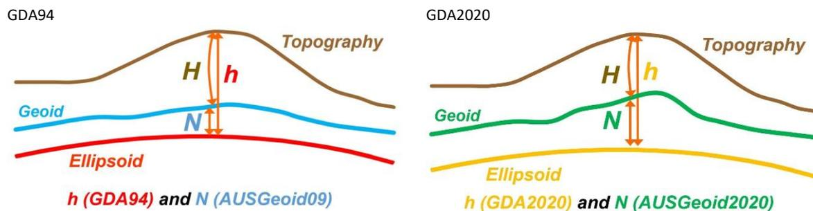
Figure 2: A difference between an ellipsoidal height based on GDA2020 and GDA94 is approximately 9 cm.
