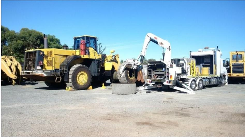
***Image 2: Vehicle mounted crane with clamp type handler attachment***
