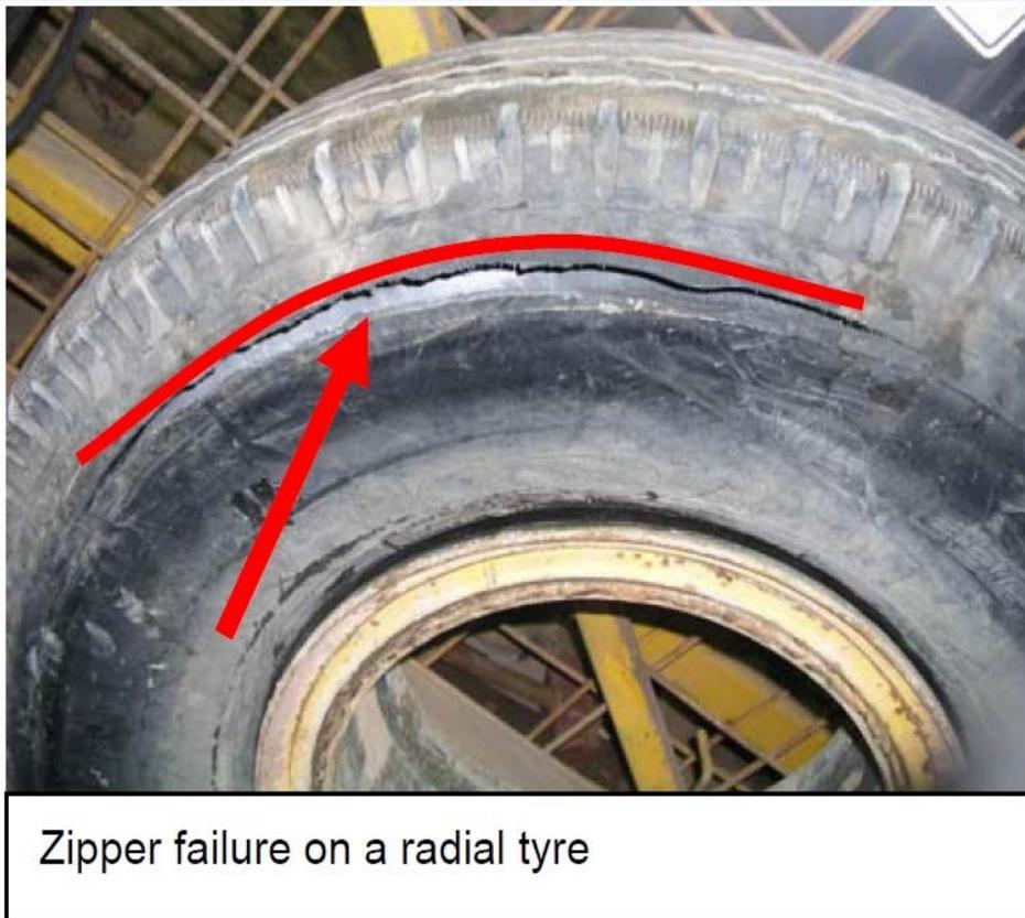
*Image 6: Zipper failure on a radial tyre*
